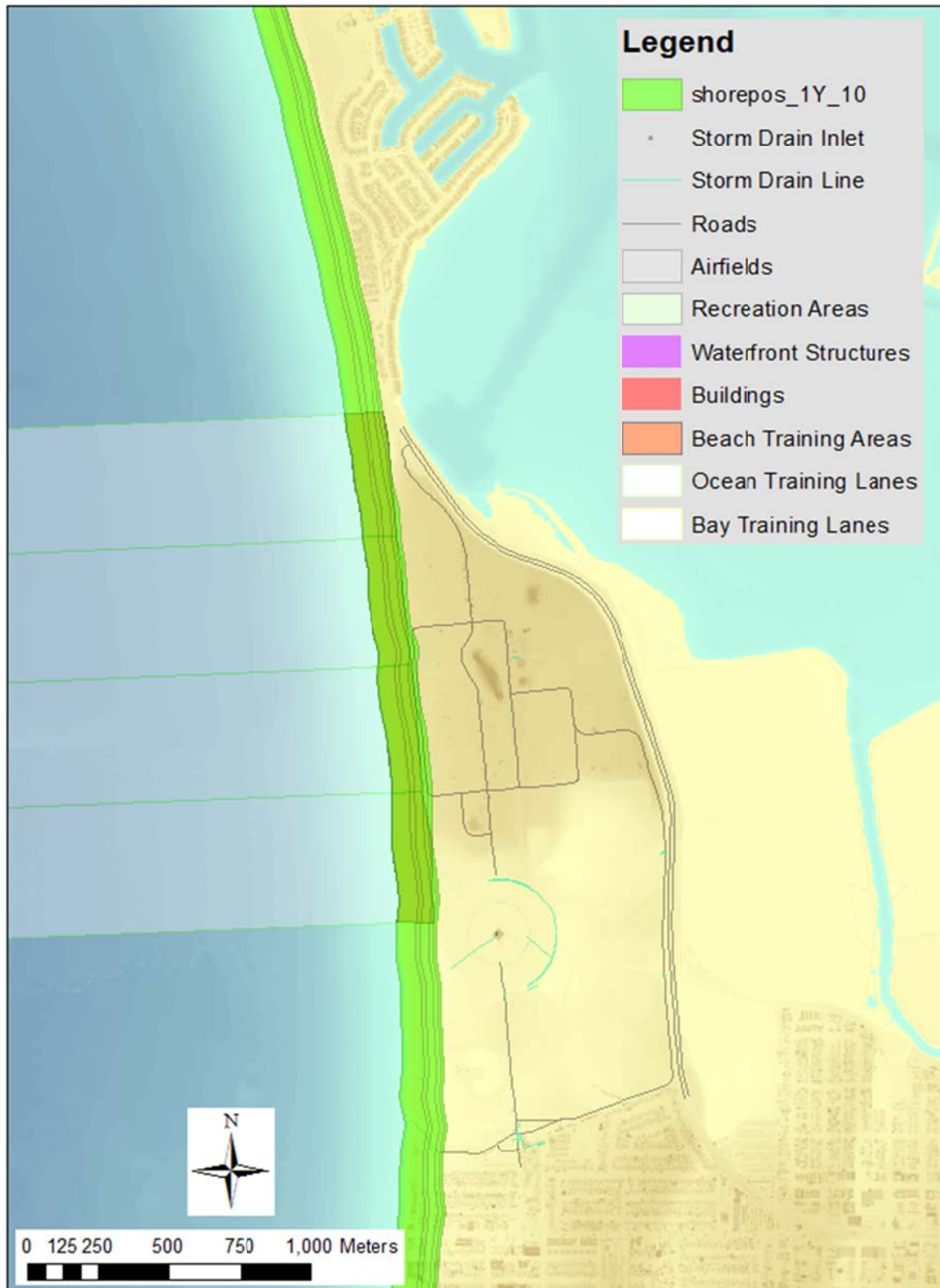
Figure 5-66. Detail view of the erosion footprint for the SLR=1.0 m scenario at SSTC South. The overall green shaded band spans the 100 year return period wave condition from the YGOR model, and the fine grey lines indicate the shorter return periods ranging from week to decade.
