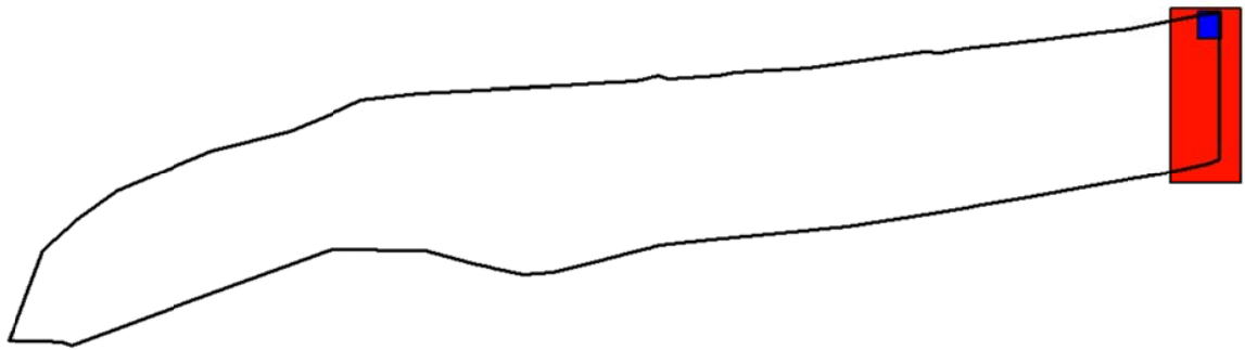
Figure 4-69. Sutra Model Element size refinement scheme. The white area has a nominal size of 5x100 m, red a nominal size of 2x40 m, and blue a nominal size of 1x20 m.
