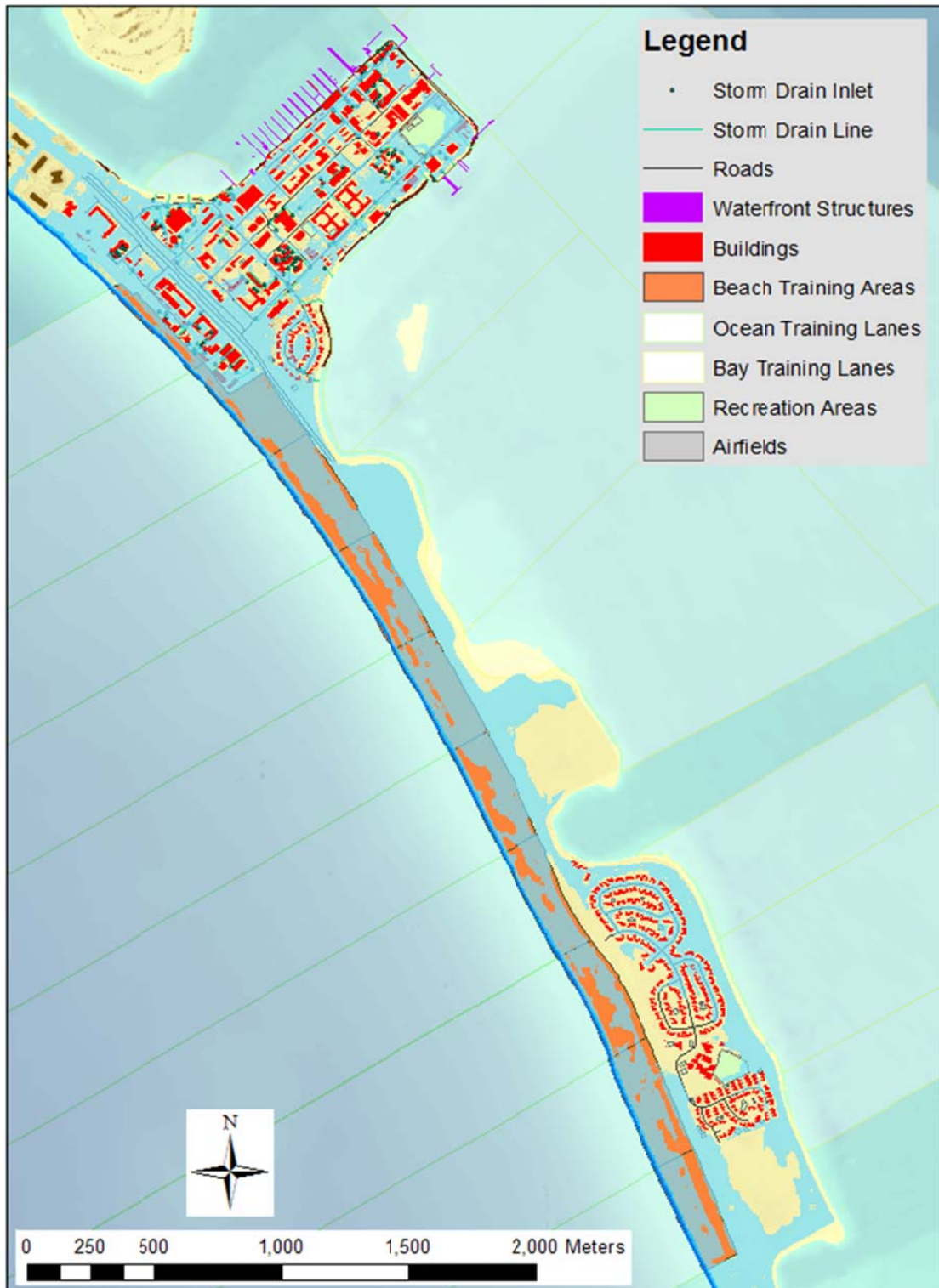
Figure 5-90. Detailed view of inundation and flooding for the baseline (SLR=0 m) scenario at NAB/STTC North. The blue shaded zones represent week (dark blue), year (medium blue) and century (light blue) return periods.
