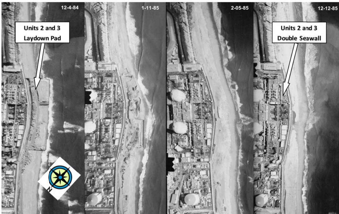
Figure 3-27. Composite of four aerial photographs of SONGS Units 2 and 3 taken near the end of construction between 4 December 1984, just before removal of the Units 2 and 3 laydown pad began (left), and 12 December 1985 (right) after beach had begun narrowing. The pad had been in place from 1974-1984. (Photos courtesy of Southern California Edison Company, see Flick et al. , 2010. Note the photo orientation with ocean on the right.)
