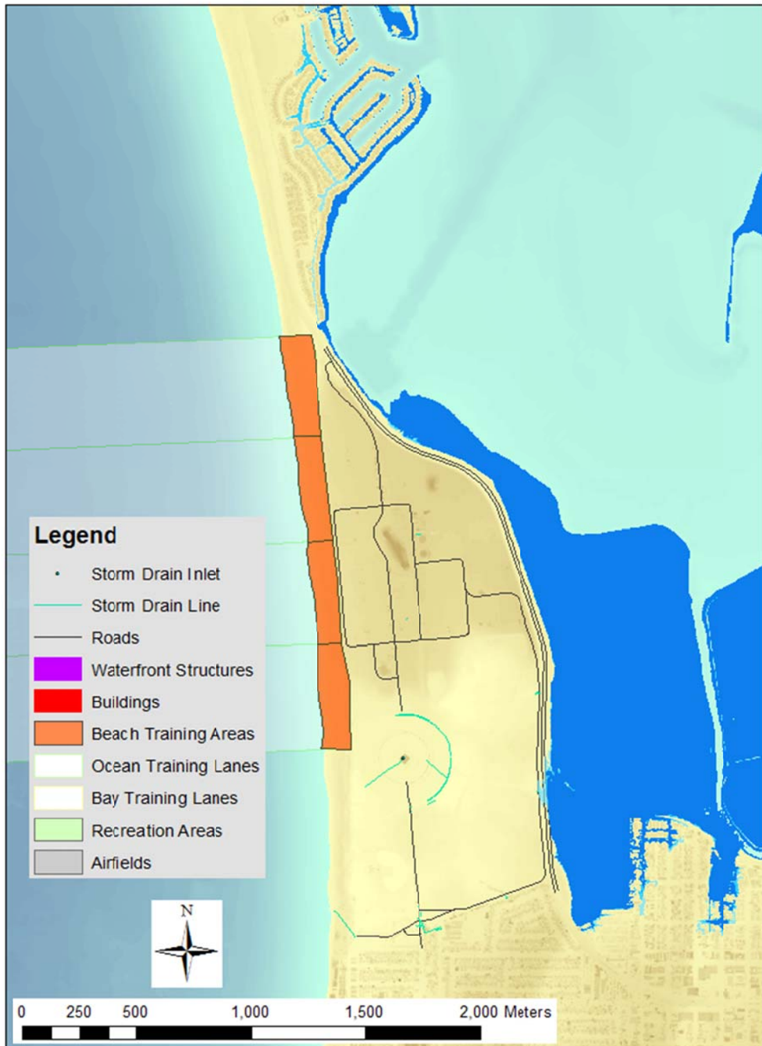
Figure 5-120. Detailed view of inundation and flooding for the 1.0 m SLR bay-exposure scenario at SSTC South. The blue shaded zones represent week (dark blue), year (medium blue) and century (light blue) return periods.
