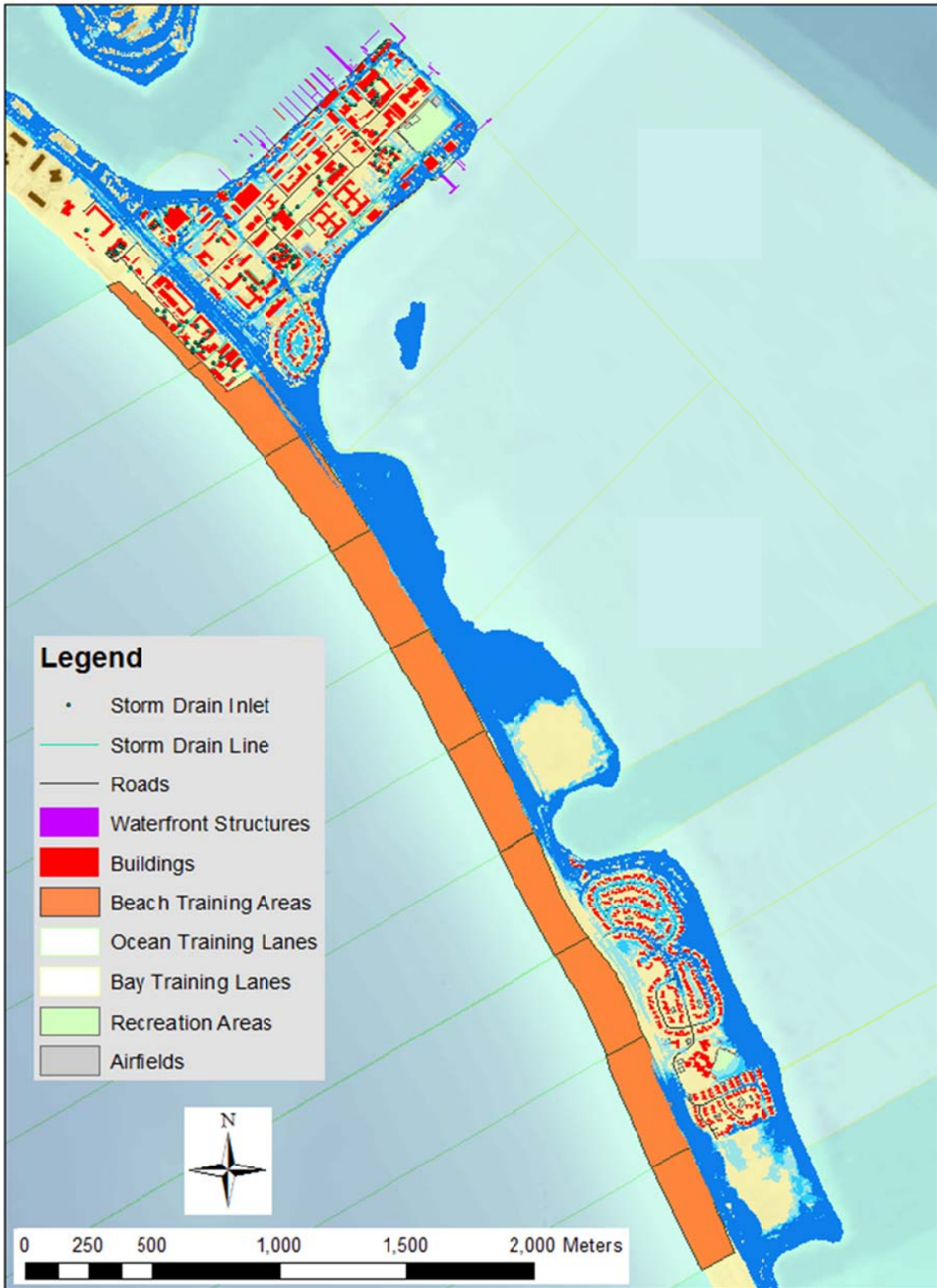
Figure 5-123. Detailed view of inundation and flooding for the 2.0 m SLR bay-exposure scenario at NAB/SSTC North. The blue shaded zones represent week (dark blue), year (medium blue) and century (light blue) return periods.
