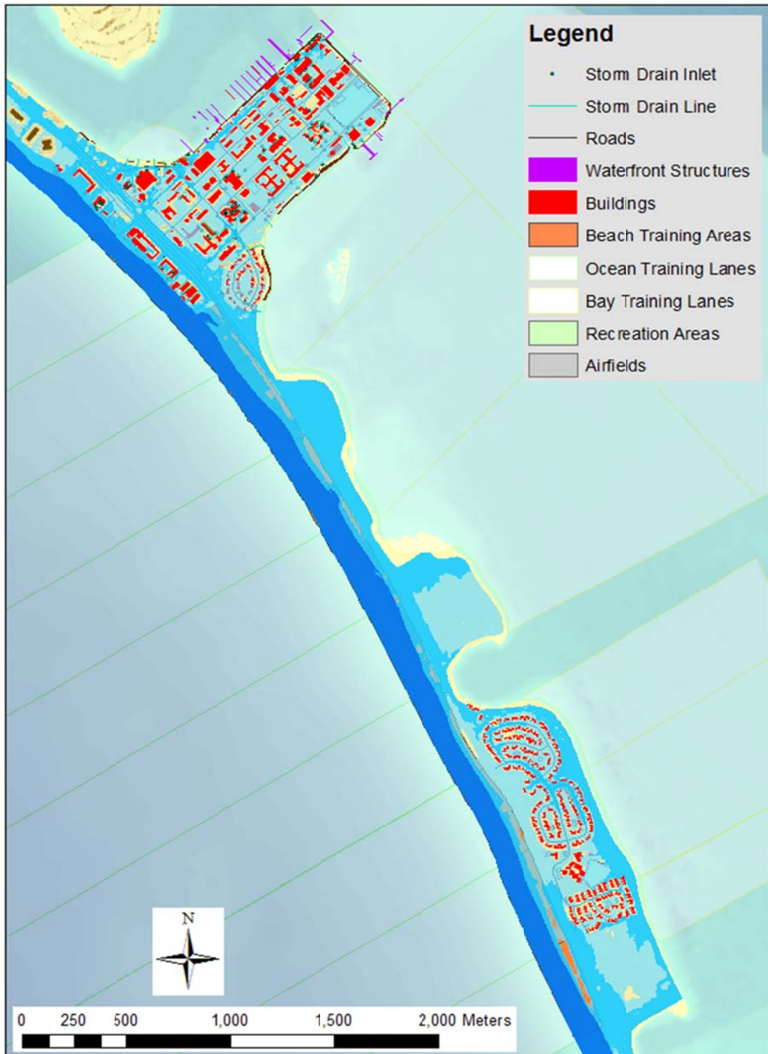
Figure 5-94. Detailed view of inundation and flooding for the SLR=1.0 m scenario at NAB/STTC North. The blue shaded zones represent week (dark blue), year (medium blue) and century (light blue) return periods.
