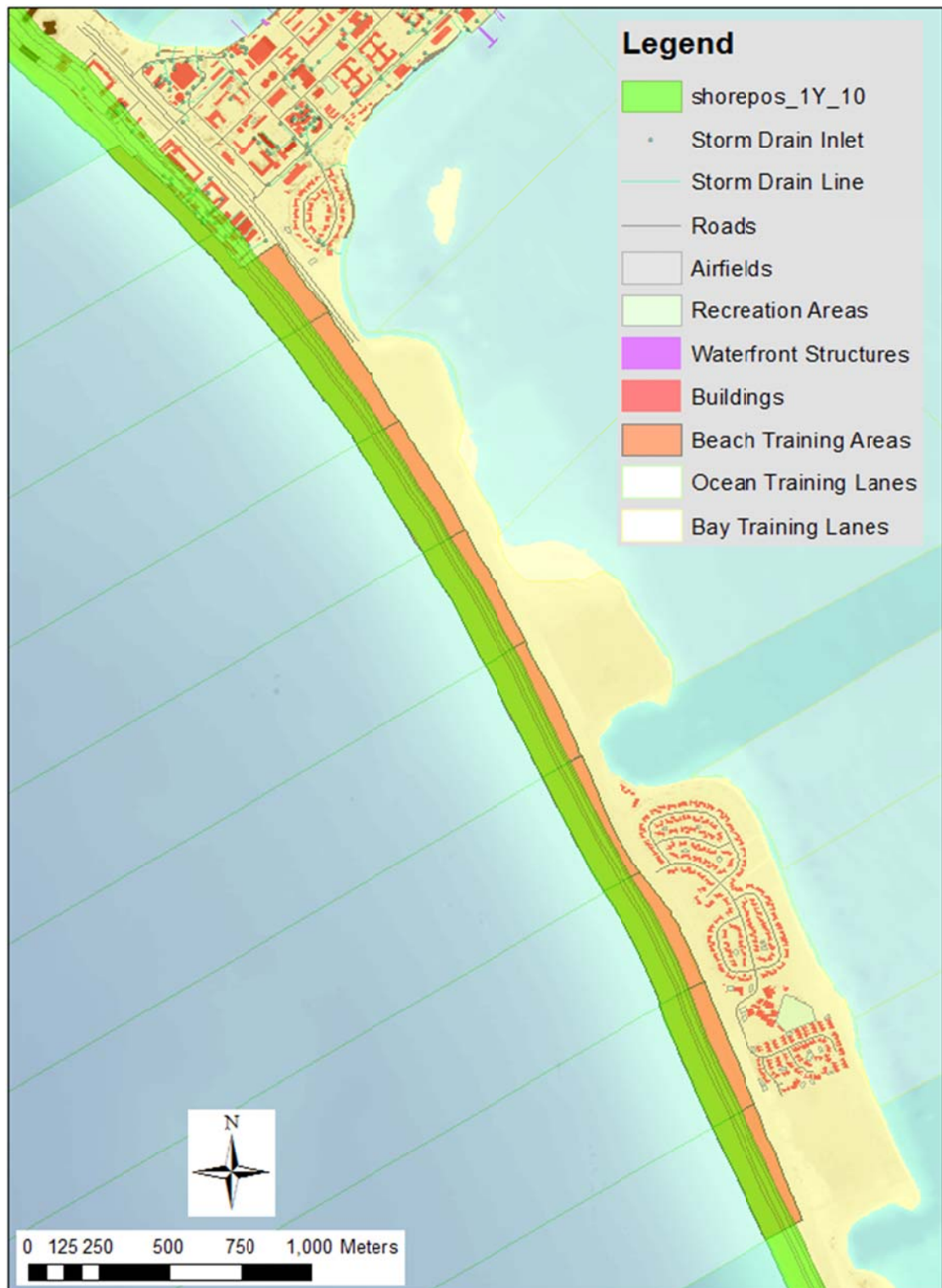
Figure 5-65. Detail view of the erosion footprint for the SLR=1.0 m scenario at NAB/SSTC North. The overall green shaded band spans the 100 year return period wave condition from the YGOR model, and the fine grey lines indicate the shorter return periods ranging from week to decade.
