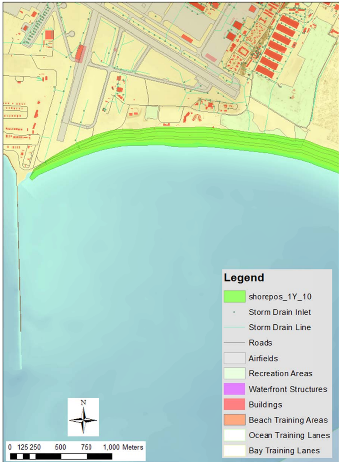
Figure 5-64. Detail view of the erosion footprint for the SLR=1.0 m scenario at North Island. The overall green shaded band spans the 100 year return period wave condition from the YGOR model, and the fine grey lines indicate the shorter return periods ranging from week to decade.
