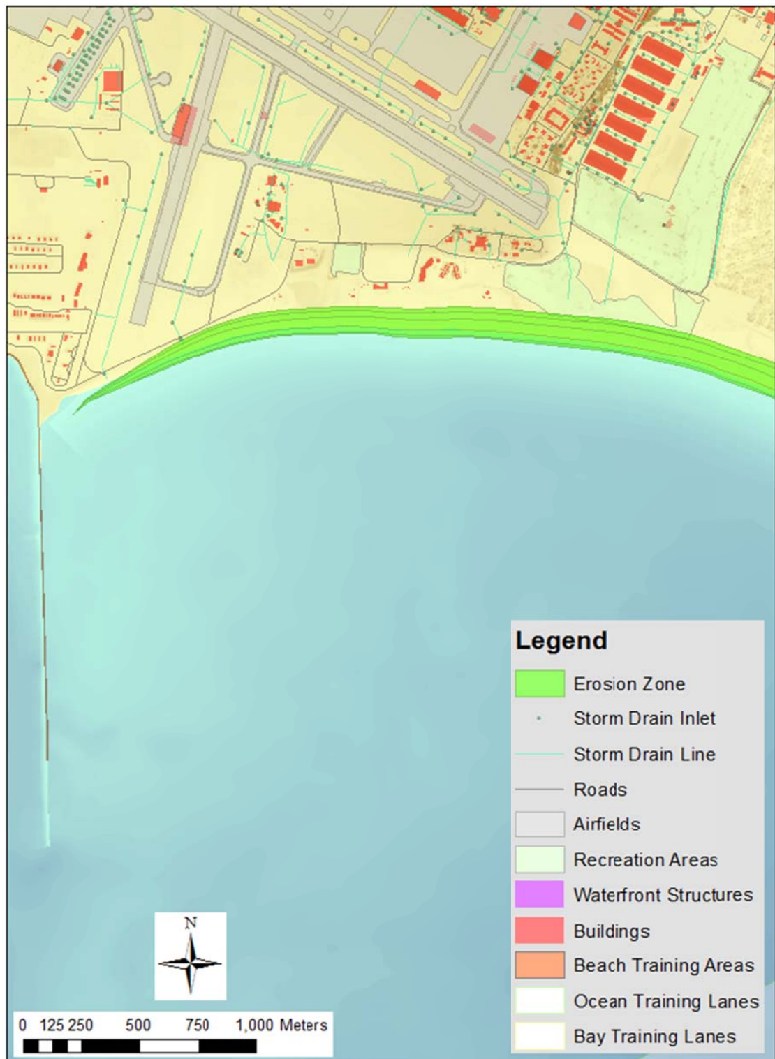
Figure 5-60. Detail view of the erosion footprint for the baseline (SLR=0 m) scenario at North Island. The overall green shaded band spans the 100 year return period wave condition from the YGOR model, and the fine grey lines indicate the shorter return periods ranging from week to decade.
