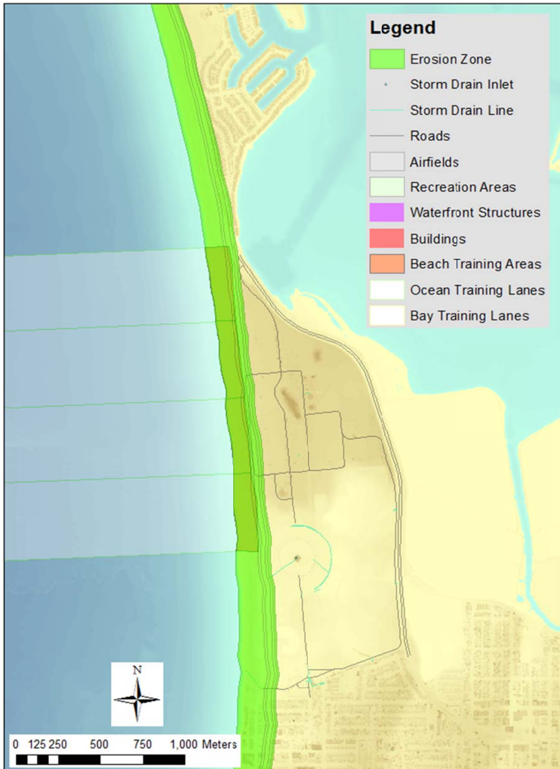
Figure 5-70. Detail view of the erosion footprint for the SLR=2.0 m scenario at SSTC South. The overall green shaded band spans the 100 year return period wave condition from the YGOR model, and the fine grey lines indicate the shorter return periods ranging from week to decade.
