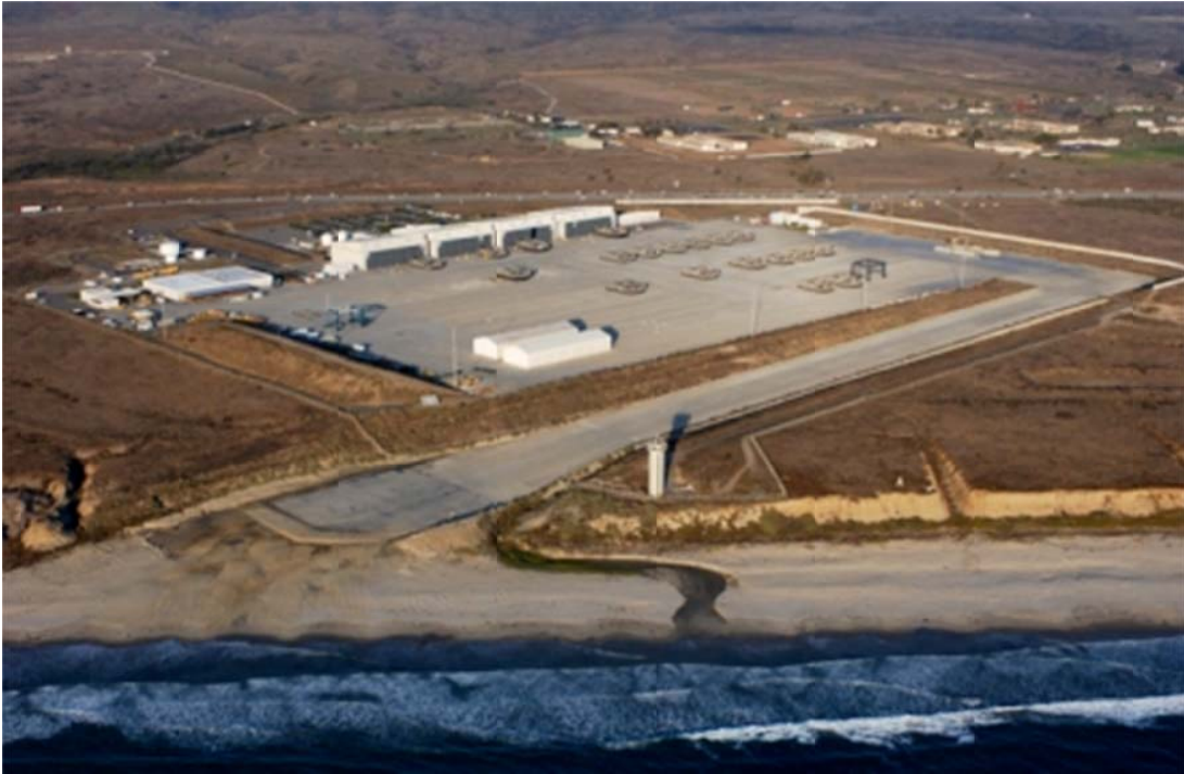
Figure 3-33. Oblique air photo of LCAC ramp taken 23 October 2004 and showing rough surface conditions at the end of the ramp, and a ditch from uncontrolled runoff (bottom center) in front of the tower (CA Coastal Records Project Image 200407314; Copyright (C) 2002-2014 Kenneth & Gabrielle Adelman, California Coastal Records Project, www.Californiacoastline.org ).
