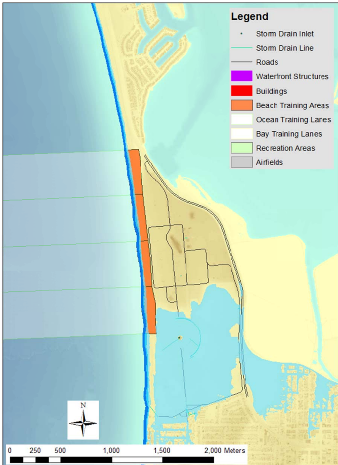
Figure 5-91. Detailed view of inundation and flooding for the baseline (SLR=0 m) scenario at STTC South. The blue shaded zones represent week (dark blue), year (medium blue) and century (light blue) return periods.
