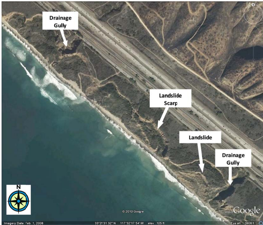
Figure 3-29. Google Earth image taken 1 February 2008 of 2 km of coast south of SONGS shows narrow, cliff-backed beach with landslides and several large gullies associated with drainage culverts and channels (see text).
