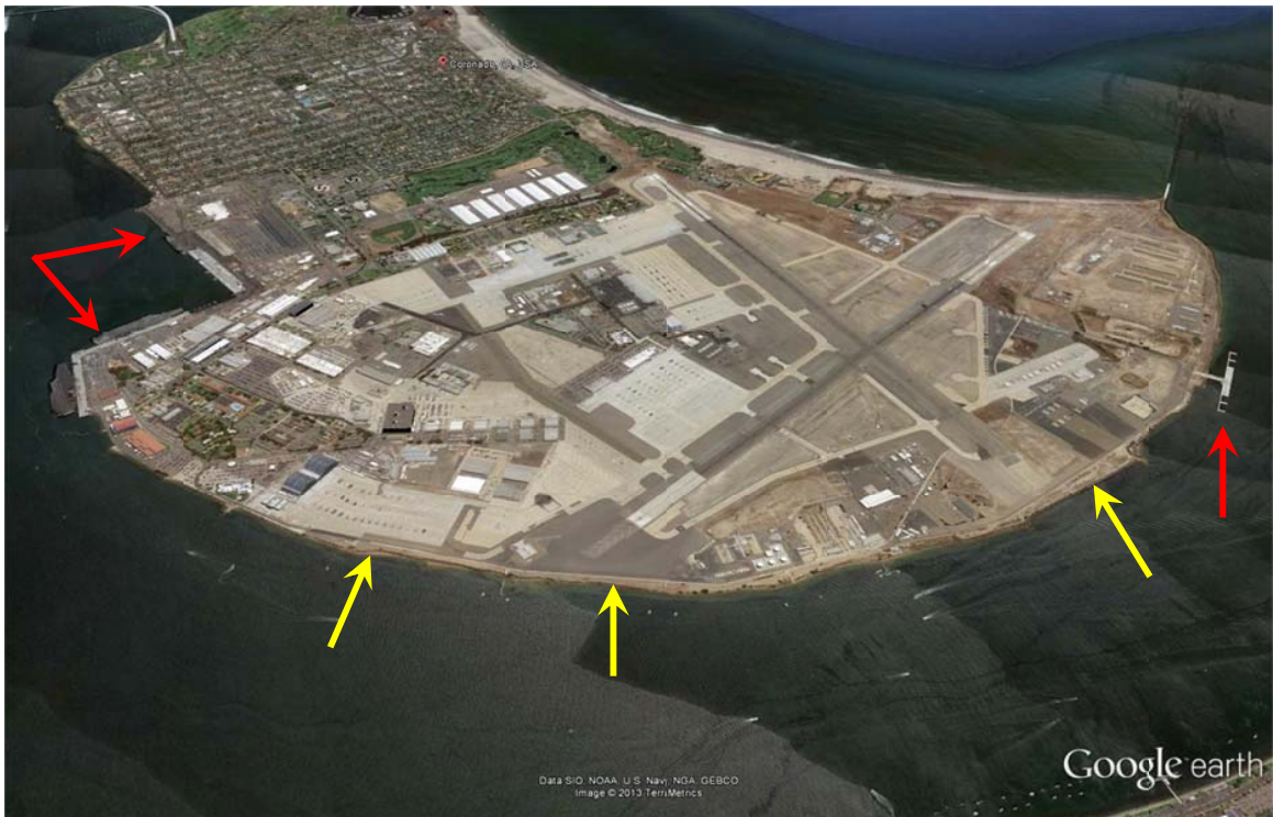
Figure 4-46. Waterfront structures at NBC including the Carrier Wharves (far left) and the Ammunition Pier (far right) (red arrows). Shore protection coastal structures can also be seen along the bay shoreline (yellow arrows) (Image data: Google).
