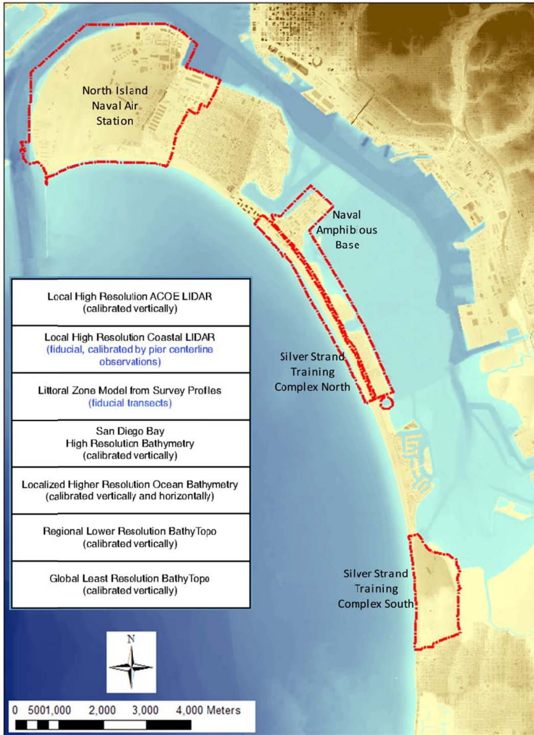
Figure 5-6. The baseline digital terrain model for NBC. Red outline show the primary areas of NBC that were evaluated in this study.
