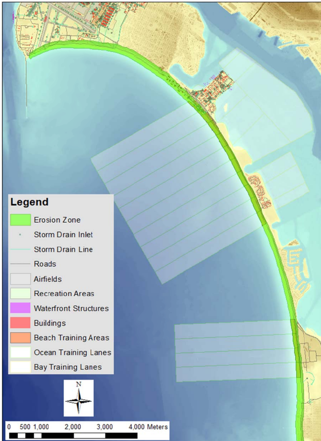
Figure 5-67. Erosion footprint for the SLR=2.0 m scenario at NBC. The overall green shaded band spans the 100 year return period wave condition from the YGOR model, and the fine grey lines indicate the shorter return periods ranging from week to decade.
