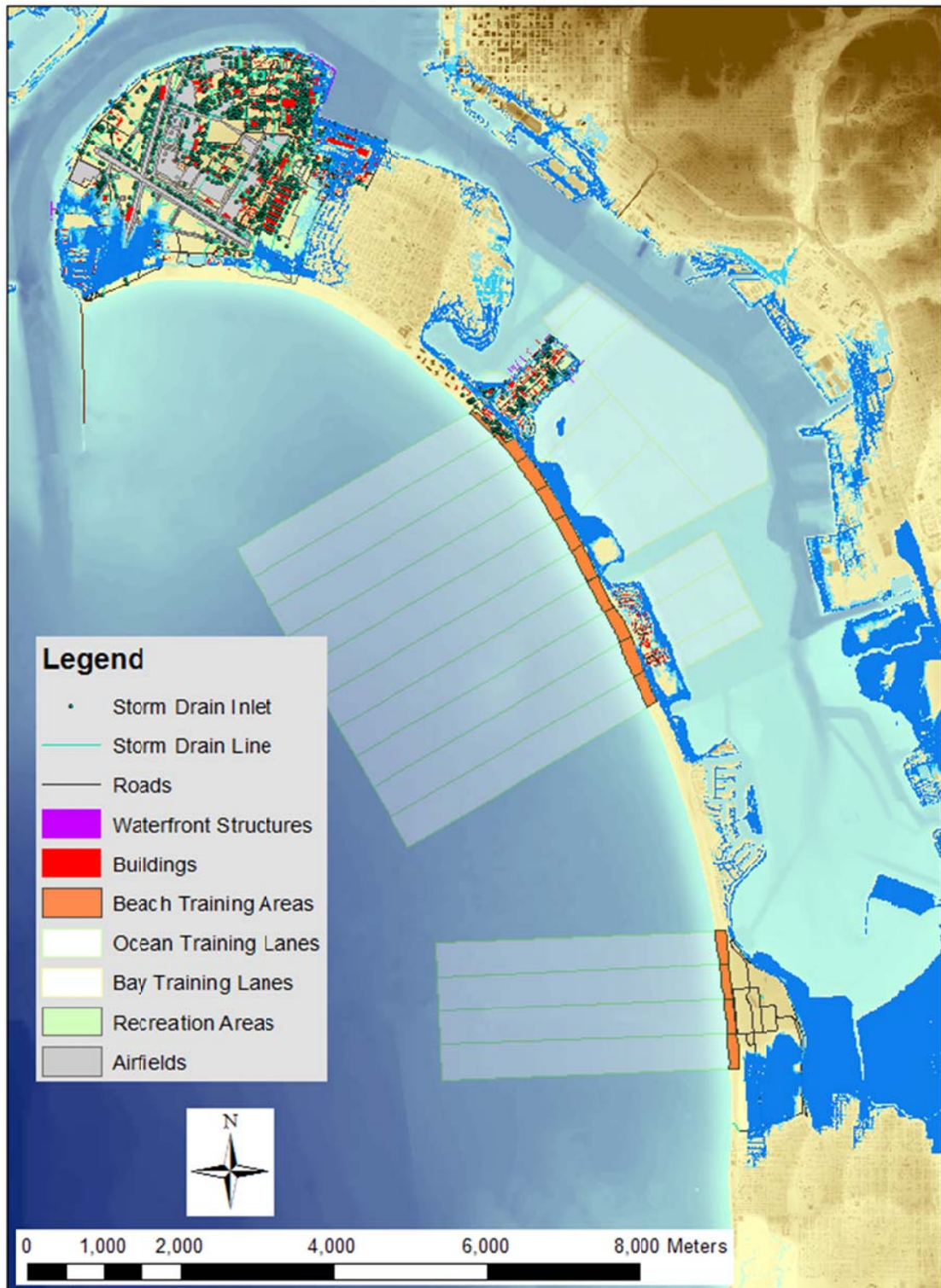
Figure 5-121. Inundation and flooding for the 2.0 m SLR bay-exposure scenario at NBC. The blue shaded zones represent week (dark blue), year (medium blue) and century (light blue) return periods.
