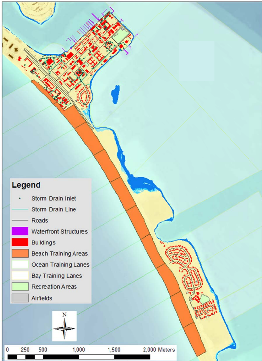
Figure 5-115. Detailed view of inundation and flooding for the baseline (SLR=0 m) bay-exposure scenario at NAB/SSTC North. The blue shaded zones represent week (dark blue), year (medium blue) and century (light blue) return periods.
