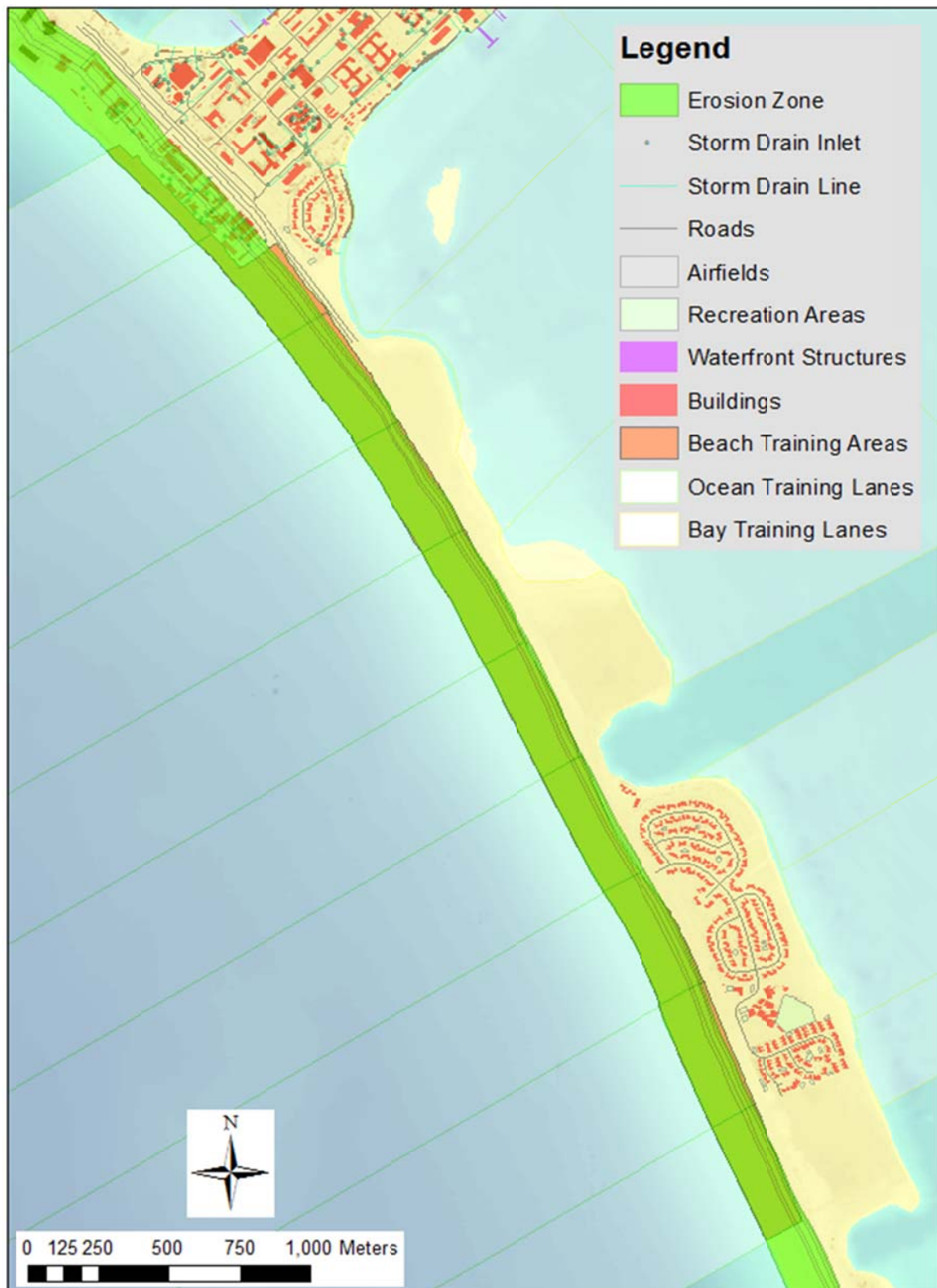
Figure 5-69. Detail view of the erosion footprint for the SLR=2.0 m scenario at NAB/SSTC North. The overall green shaded band spans the 100 year return period wave condition from the YGOR model, and the fine grey lines indicate the shorter return periods ranging from week to decade.
