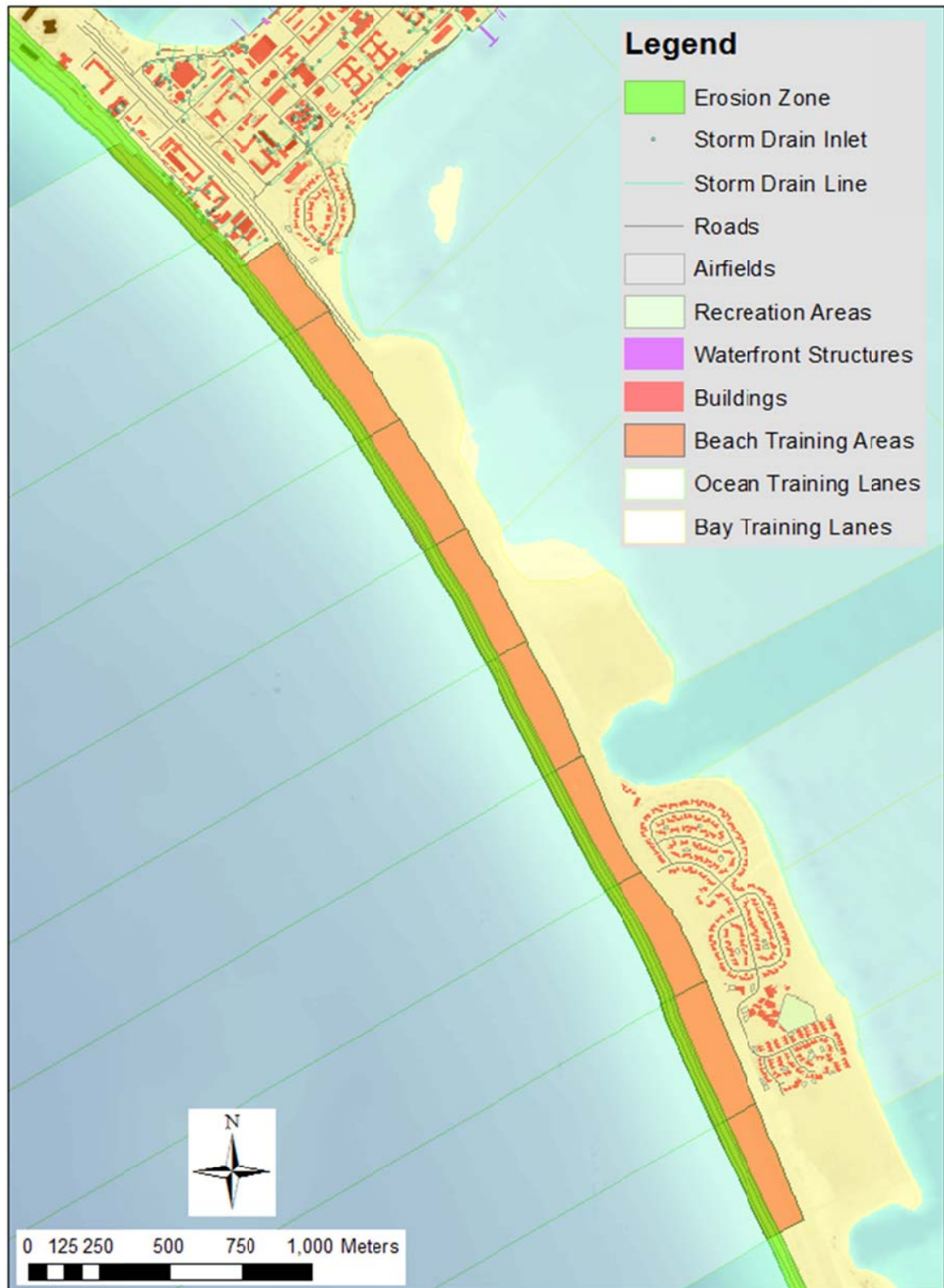
Figure 5-61. Detail view of the erosion footprint for the baseline (SLR=0 m) scenario at NAB/SSTC North. The overall green shaded band spans the 100 year return period wave condition from the YGOR model, and the fine grey lines indicate the shorter return periods ranging from week to decade.
