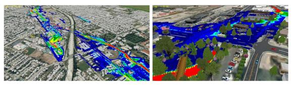
Graphic results of 2-dimensional flood routing analysis used to develop the City's master plan update
