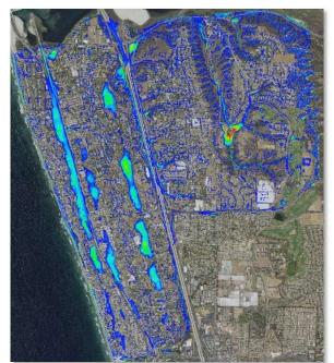
Leucadia WS - XPSTORM (2D Only Test Run) used to Identify potential Bifurcation
